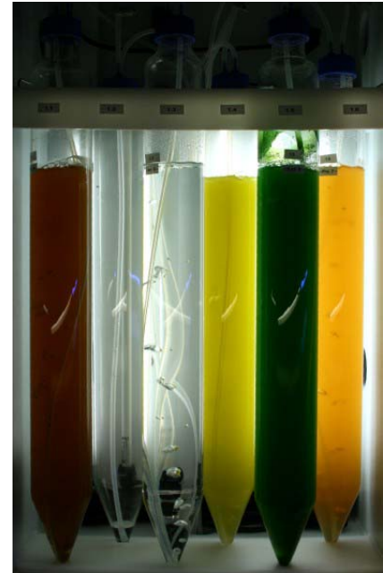
Algae tubes with minimum 4 liters (1 US gal) volume are the minimum for breeding algae for zooplankton picture: AquaCare
