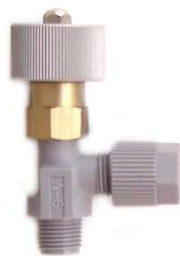
grinded flushing valve: in the closed position the right concentrate flow is established. Every membrane size need its specific flushing valve.
