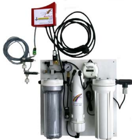
Reverse osmosis unit with R.O. control (automatically re-filling and flushing function), ultra pure water filter and ultra pure water conductivity meter.
