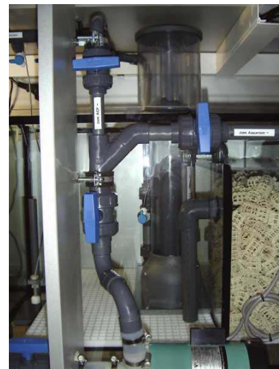
orderly laid tubes ensure a maximum amount of safety and lettering of the tubes ensures the usability by hobbyists. Picture: AquaCare.
