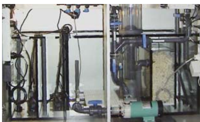
Filter tank, refill tank and mixing tank made of glass for a sea water aquarium. Picture: AquaCare.
