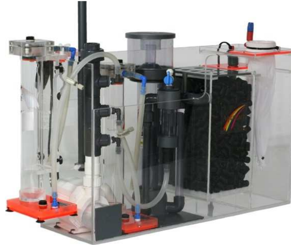
Basic 70 filter system with exemplary filter technology: heater, measuring chains for pH and ORP, skimmer ACF300A, 2 × empty filter MF 2 -50, energy-saving pump for quiet operation and economical use
