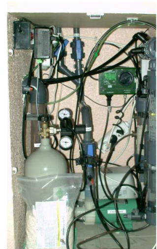
Basic 70 filter system with exemplary filter technology: heater, measuring chains for pH and ORP, skimmer ACF300A, 2 × empty filter MF 2 -50, energy-saving pump for quiet operation and economical use
