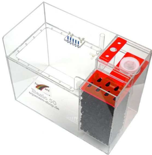
Filter system Basic 50 made of acrylic glass (Plexiglas) in the basic configuration with Inlet chamber, sock filter, heater holder, degassing chamber, float valve and hose holder
