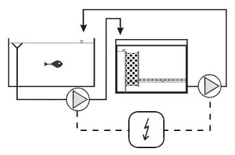
This variant is only suitable with a costly electronic. Without an electronic level control it is not possible to synchronize two pumps permanently.
