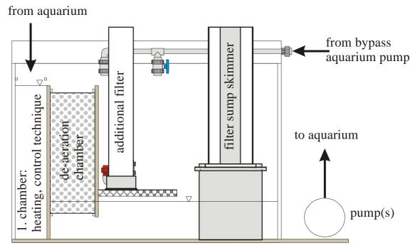
The unit is made from rigid PE plates and PE hollow chamber plates:
