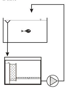
Normally the aquarium is over the filters system. The water flow from the aquarium overflow downwards into the filter system. At the outlet of the *Basic* a circulation pump pushes the water back to the aquarium.
